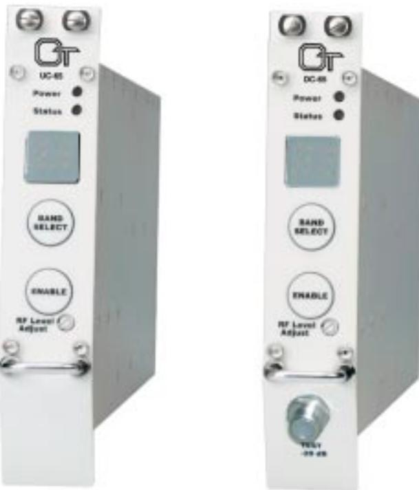
The **OTMS-II TWELVE-BAND MULTIPLEX SYSTEM** is made up of three key units. they consist of an up-converter model **UC-65**, that multiplexes up to twelve 5MHz to 65MHz return bands into one fiber or coaxial in the frequency band of 4.5MHz to 875MHz, a down-converter model **DC-65** that de-multiplexes the combined band into twelve 5MHz to 65MHz outputs, and the model **OTMS-II** Mainframe that acts as a common platform for both the downstream / upstream converters.
