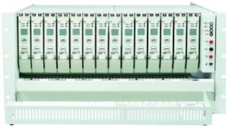
The **OTMS-II MAINFRAME**, model **OTMS-II**, makes efficient use of rack space ( 8.75”H x 19”W x 20”D ) while housing, powering and routing status information between the up-converter and down-converter modules of the Multiplex System. It is a common platform for both the downstream / downstream modules. Several power systems are available. Although fans, blowers, and rack spacers are not usually required.
