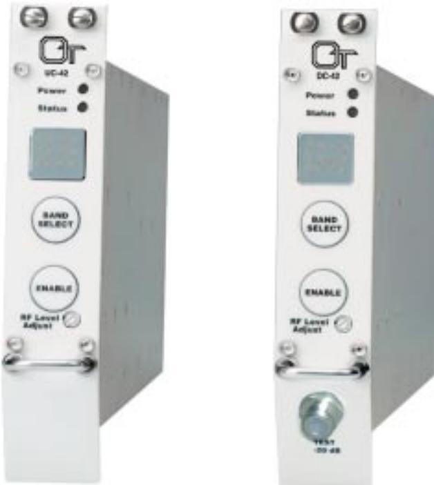
The **Eighteen-Band (5 to 42MHz) Converter System** is made up of three key units. They consist of an up-converter model **UC-42** that multiplexes up to eighteen 5MHz to 42MHz return bands into one fiber or coaxial in the frequency band of 4.5MHz to 883.5MHz, a down-converter model **DC-42**, that de-multiplexes the combined band into eighteen 5 to 42MHz outputs, and the model **OTMS-II** Mainframe that acts as a common platform for both the downstream / upstream converters.
